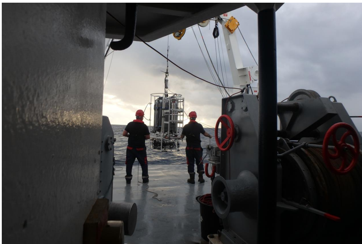
Deployment of the CTD Rosette with UVP at the DYFAMED site from the deck of the R/V Téthys II
